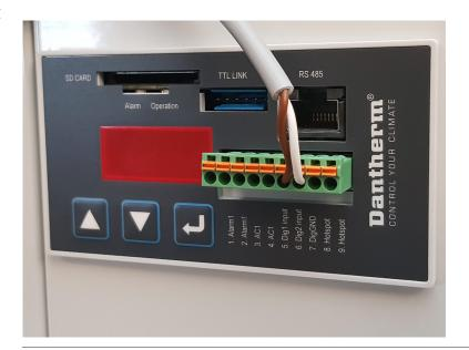
Pin 6: Digital 2 input pin 7: Digital Ground.
